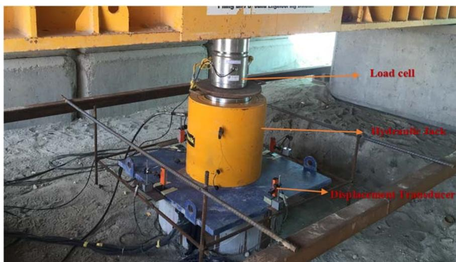
**Picture (2): CFA pile test setup**
