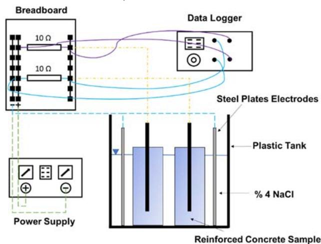
Figure (5): Schematic representation of accelerated corrosion test
