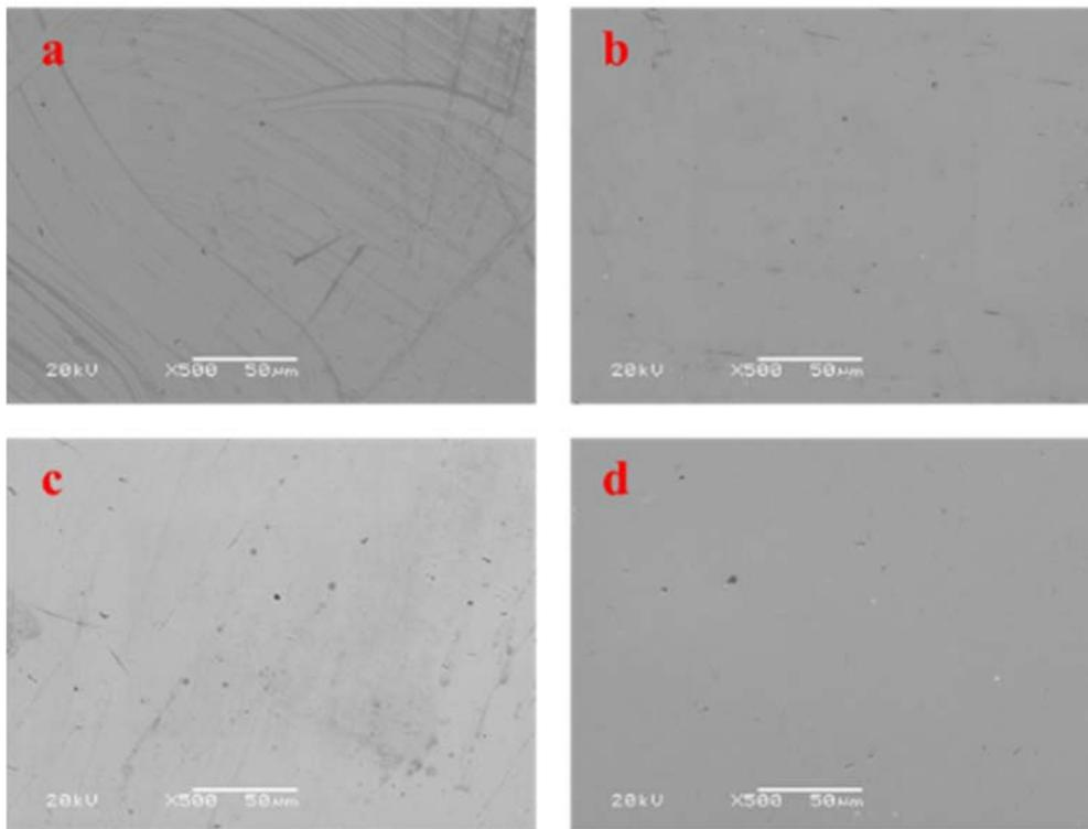
Figure (7): SEM analysis for (a) un-coated, (b) Ti, (c) TiO<sub>2</sub> and (d) TiB<sub>2</sub> nano-coated samples
