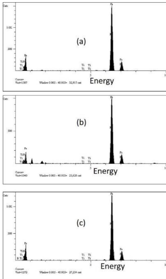
**Figure (8): EDX analysis spectrum of rebar samples coated with (a) Ti, (b) TiO<sub>2</sub> and (c) TiB<sub>2</sub>**
