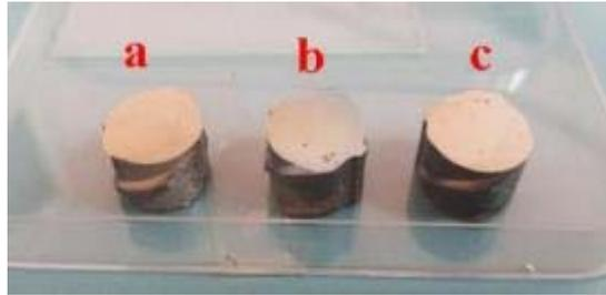
Figure (6): (a) Ti, (b) TiO<sub>2</sub> and (c) TiB<sub>2</sub> nano-coated rebars for surface analysis
