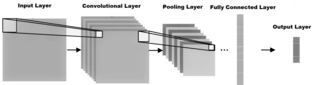
Figure (2): Basic structure of convolutional neural network
