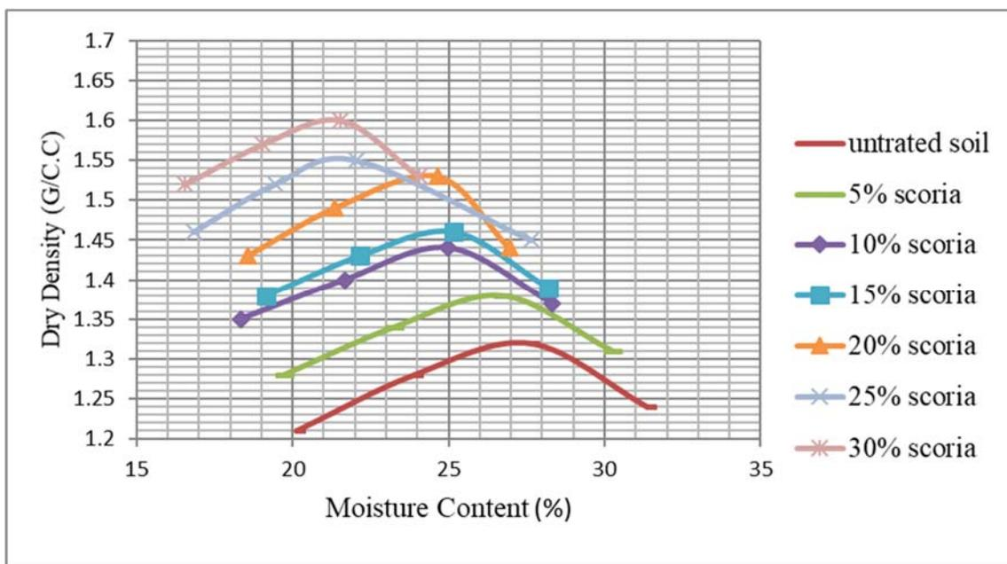
Figure (5): The effect of scoria on the compaction of the soil
