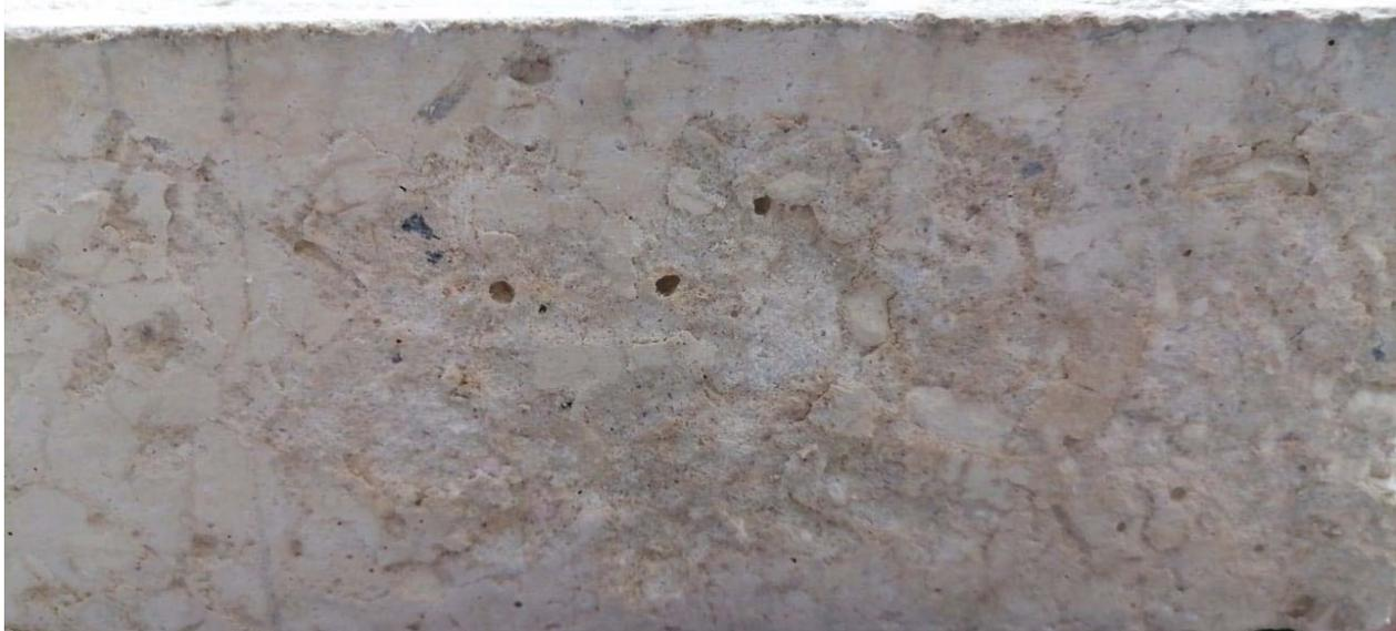
(b) Concrete specimen with 75% SSA
