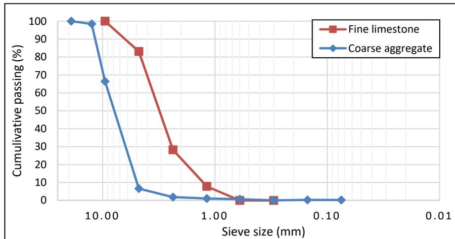
**Figure (1): The coarse and fine aggregate gradients**
