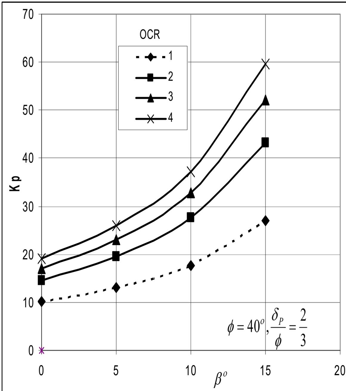
Figure (8): Coefficient of passive earth pressure for inclined homogeneous normally and
