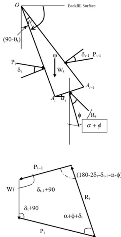
Figure (3): Slice forces' hodograph for a typical slice ( $i$ )
