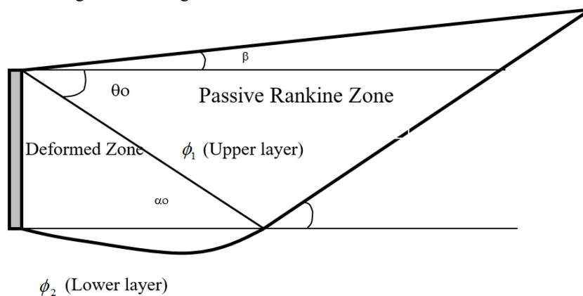
Figure (5): Failure plane for inclined backfill material of an angle behind a retaining wall
