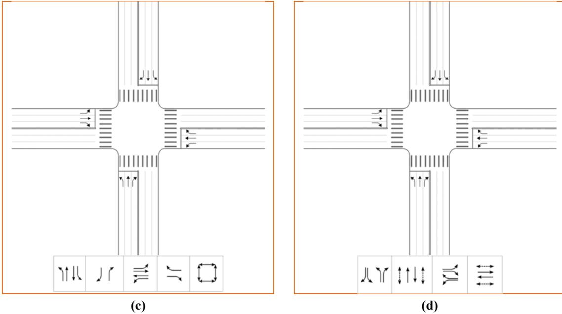
**Figure 4): (a) ACD-1: ACD with same cycles at intersection and mid-block crosswalks, (b) ACD-2: ACD with half cycle at mid-block crosswalks, (c) TCD-1: Traditional crosswalk design with exclusive pedestrian phasing scheme and (d) TCD-2: Traditional crosswalk design with concurrent pedestrian phasing scheme**
