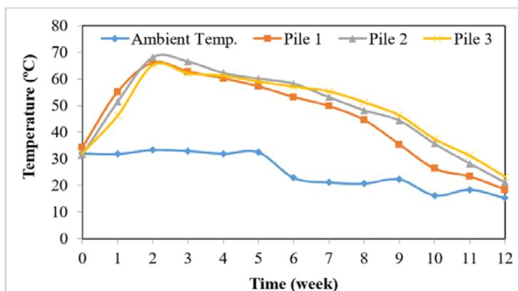
**Figure (1): Temperature profiles for piles and ambient temperature during the composting process**
