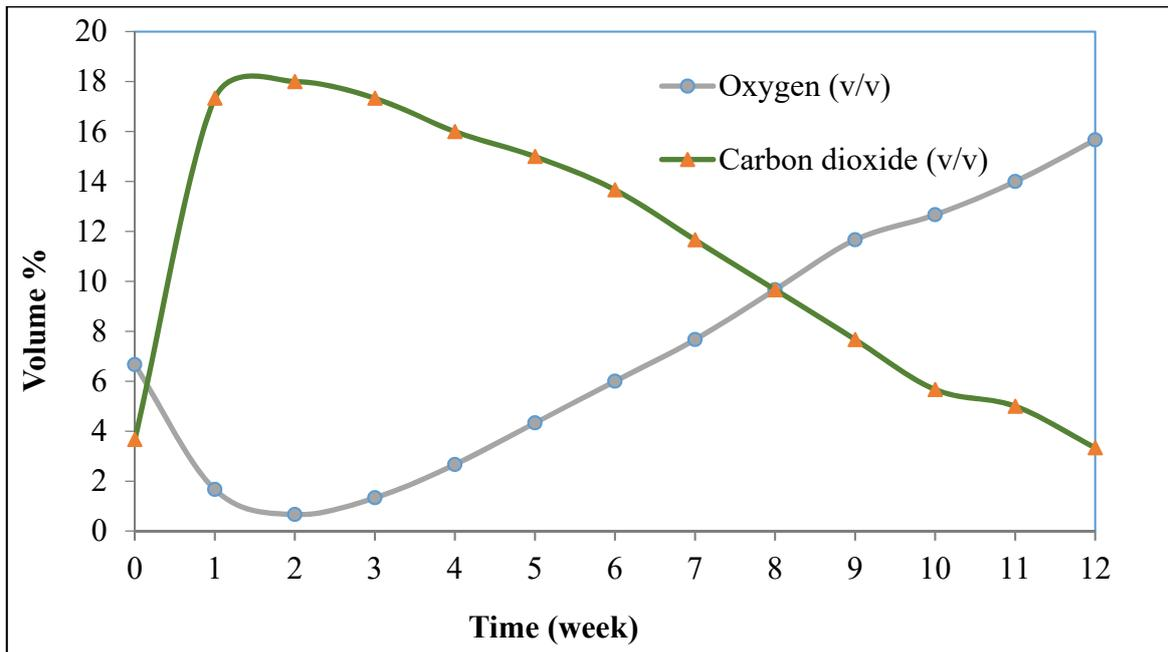
Figure (2): O<sub>2</sub> and CO<sub>2</sub> concentrations for pile 2 during composting period
