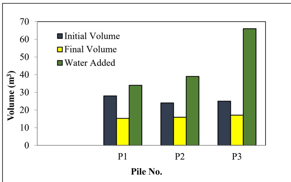
Figure (4): Volume of piles and water consumption
