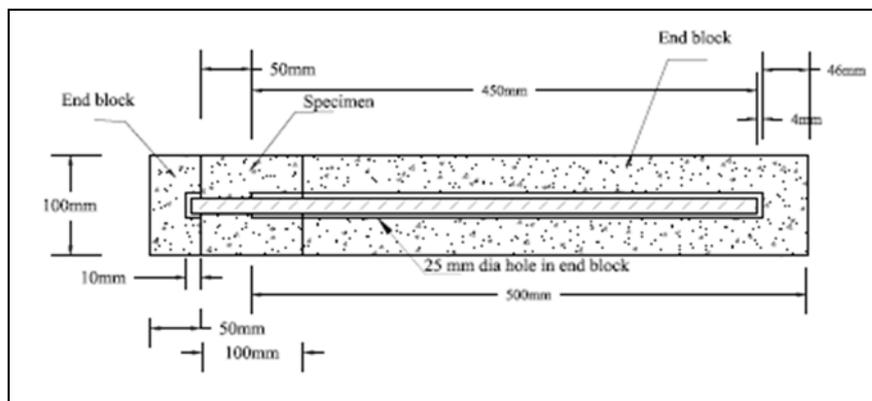
Figure (3): Assembly of a pull-out specimen with end blocks
