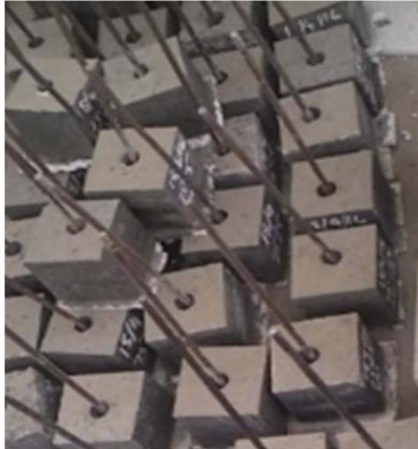
Figure (2): Pull-out specimens
