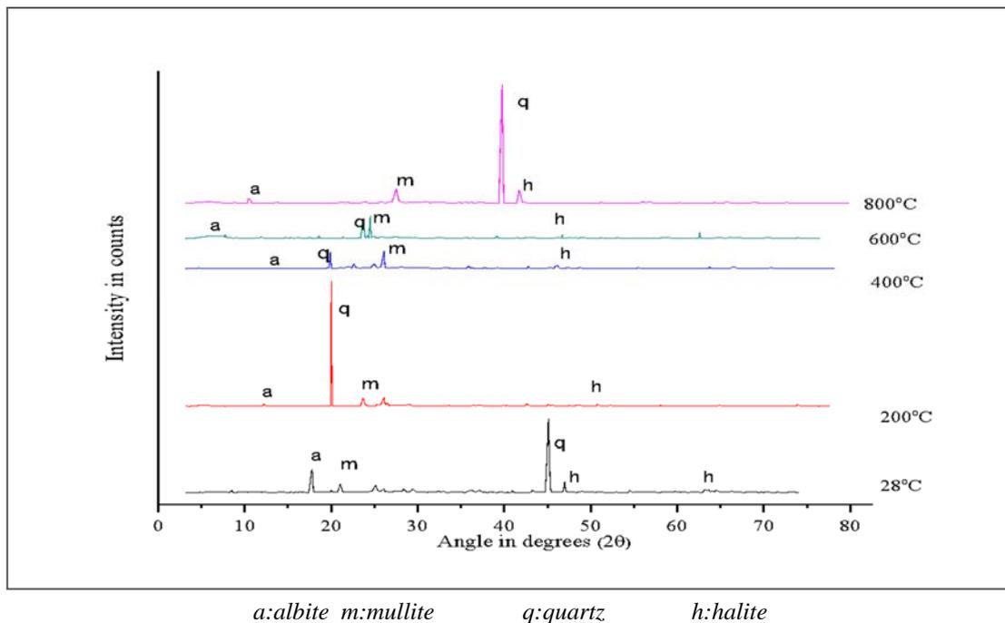
Figure (9): Typical XRD diffractogram of geopolymer concrete (F50GPNA)
