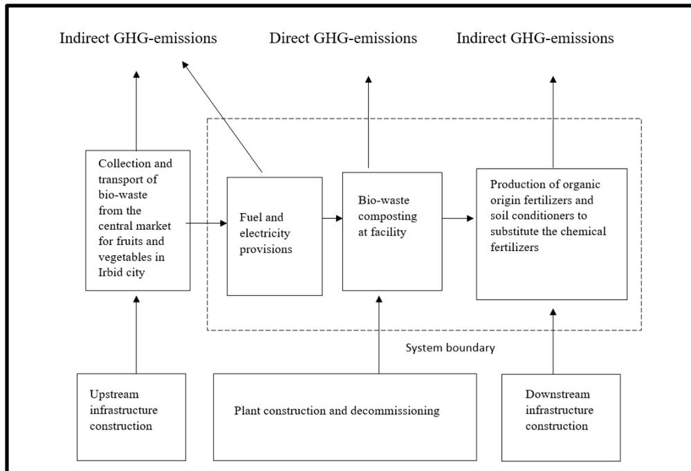
**Figure (2): Model conceptual framework showing the system boundaries, upstream and downstream processes (Abu Qdais et al., 2019)**
