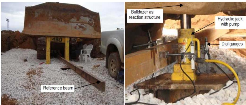
Figure (6): Load test on stone column
