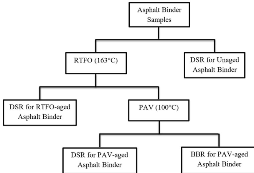
**Figure (1): PG grading flowchart**
