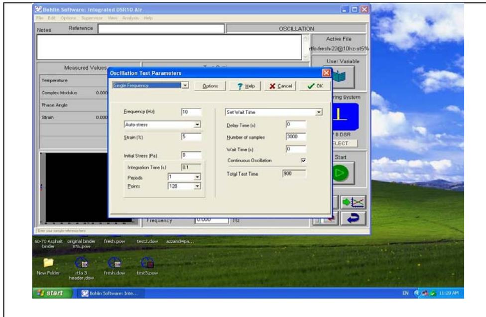
**Figure (2): Setting parameters for the DSR test**
