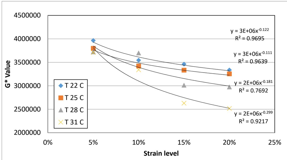
Figure (12): Effect of temperature on complex modulus for PAV60-aged unmodified asphalt
