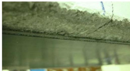
Figure (5): Intermediate crack induced in the adhesive layer (Fayyadh and Razak, 2012)
