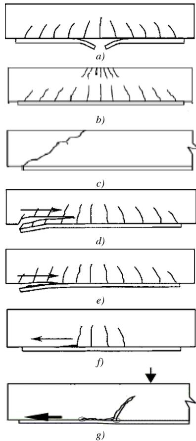
**Figure (4): Failure modes of FRP flexural strengthening or repair [a) FRP rupture, b) Concrete crushing, c) Shear failure, d) Concrete cover separation, e) Plate end interfacial debonding, f) Flexural crack-induced interfacial debonding, g) Flexural-shear crack-induced interfacial debonding] (Ritchie et al., 1991; Saadatmanesh and Ehsani, 1991; Triantafillou and Plevris, 1992; Sharif et al., 1994; Chajes et al., 1994; Heffernan and Erik, 1996)**
