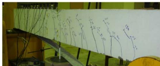
Figure (6): Crack pattern and failure mode (Fayyadh and Razak, 2012)
