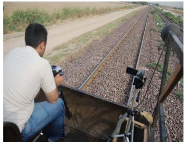
Figure (7): Track survey by car and camera (Tehran-GARMSAR), train speed of 20 to 30 km/h
