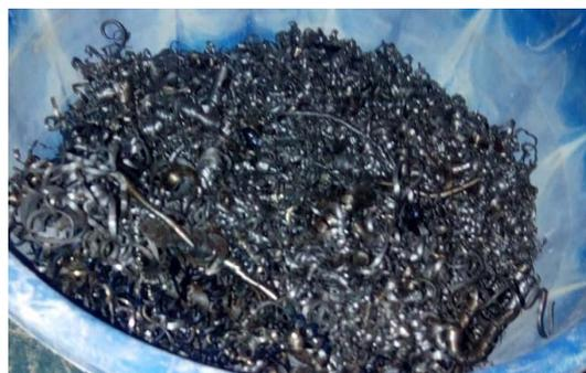
Figure (2): Lathe waste steel fiber
