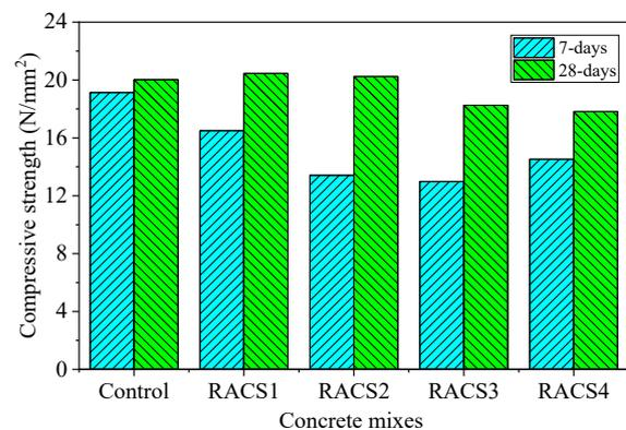
Figure (4): Compressive strength at 7 days and 28 days for different concrete mixes
