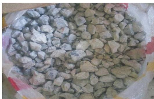
Figure (1): RCA (laboratory-tested samples)
