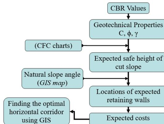
Figure (10): Flowchart of using retaining wall costs in extracting the horizontal road corridor using GIS
