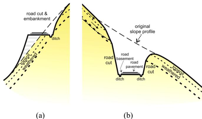
Figures (4): Roadside retaining walls in a mountainous terrain: (a) road cut and embankment; (b) road cuts
