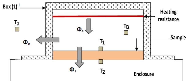
Figure (3): Thermal conductivity testing device
