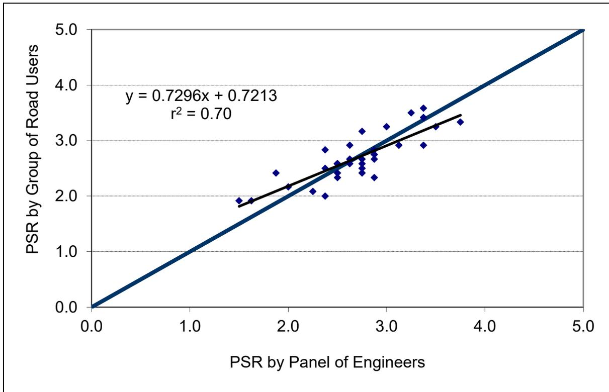
Figure (2): PSR by panel of engineers vs. PSR by group of road users
