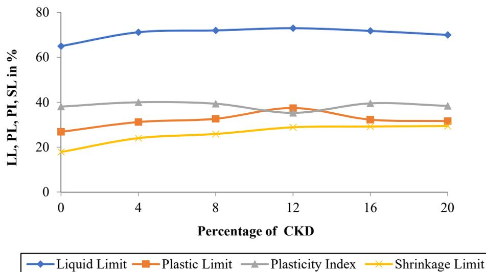
Figure (1): Variation of plasticity characteristics of CKD-admixed BC soil
