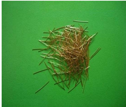
Plate (1): Copper-coated steel fibers
