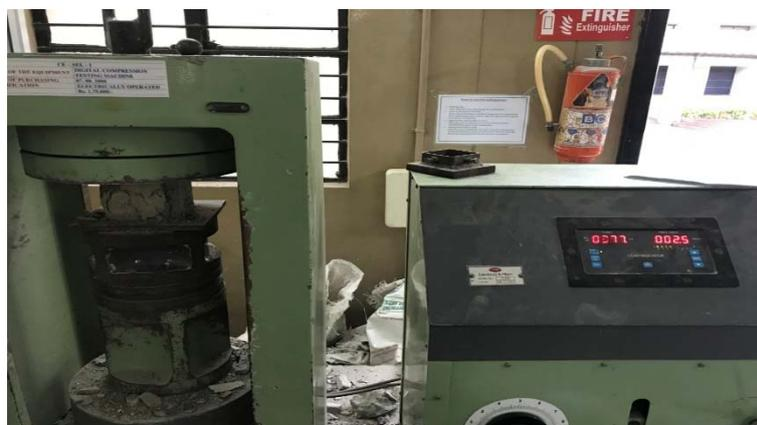
**Figure (3): Compressive strength test**
