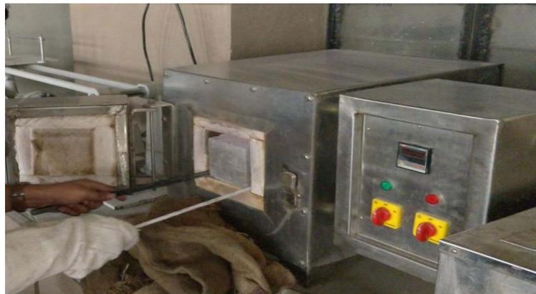
**Figure (2): Specimens kept at elevated temperatures**
