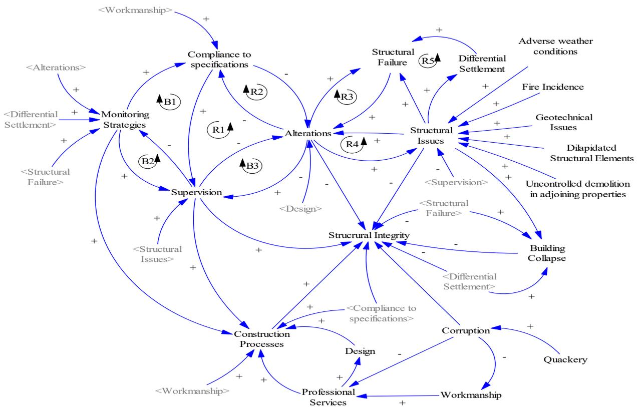
Figure (3): Causal loop diagram for building collapse in Nigeria
