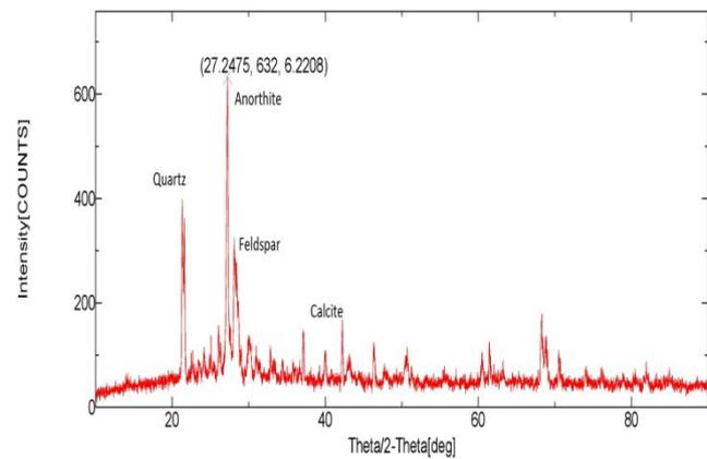
**Figure (4): X-ray diffraction pattern of optimized quaternary blended concrete mix**
