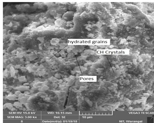
**Figure (6): SEM image of cement hydration for optimized quaternary blended SCM mix**
