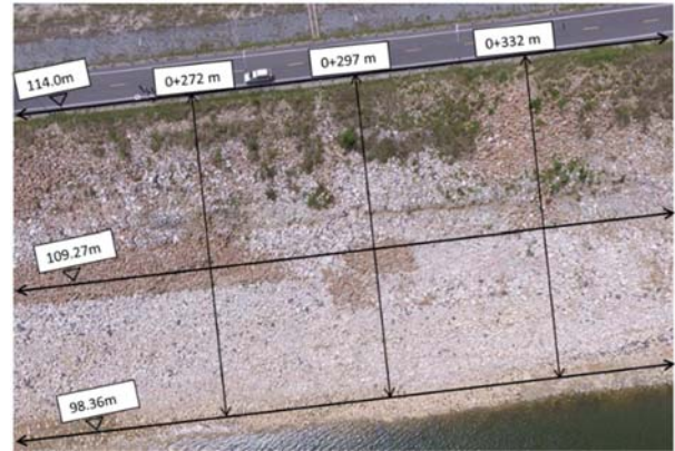
Figure (11): Location for the conduction of electrical resistivity test
