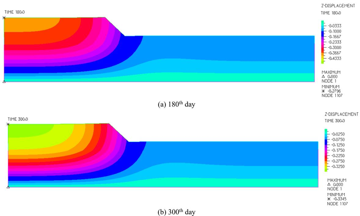
**Figure (11): Settlement nephogram of the high embankment**
