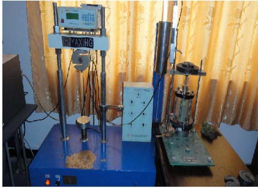
Figure (1): Modified triaxial creep equipment
