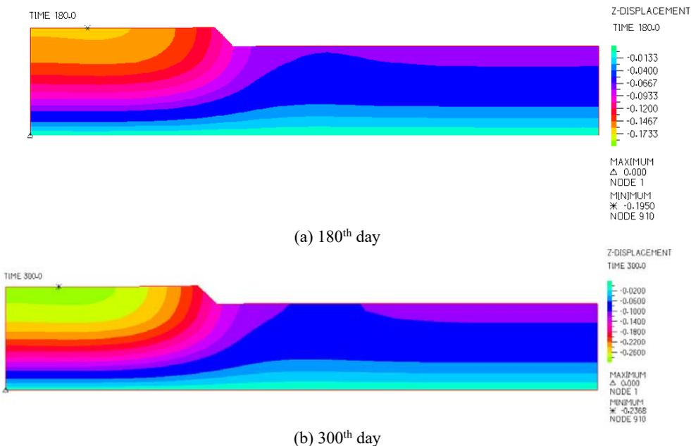
**Figure (10): Settlement nephogram of the low embankment**
