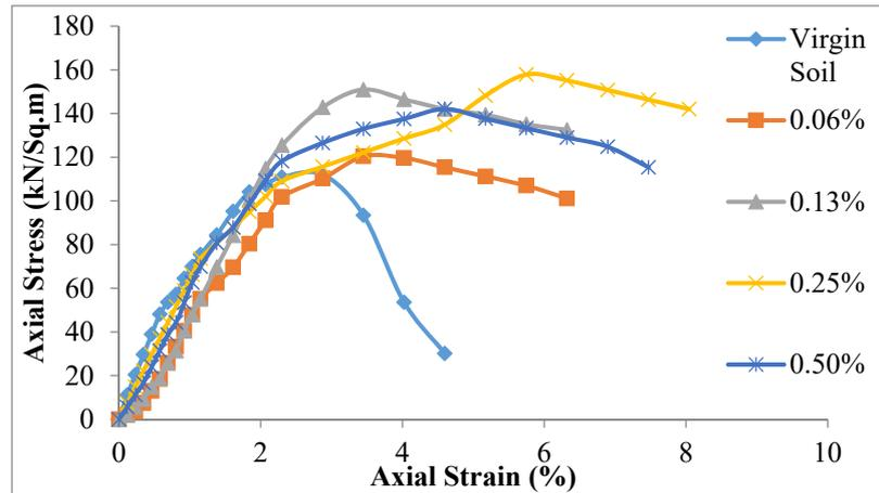
Figure (5): Axial stress-strain curves for unreinforced and kenaf fibre-reinforced Karwi (clayey) soil specimen
