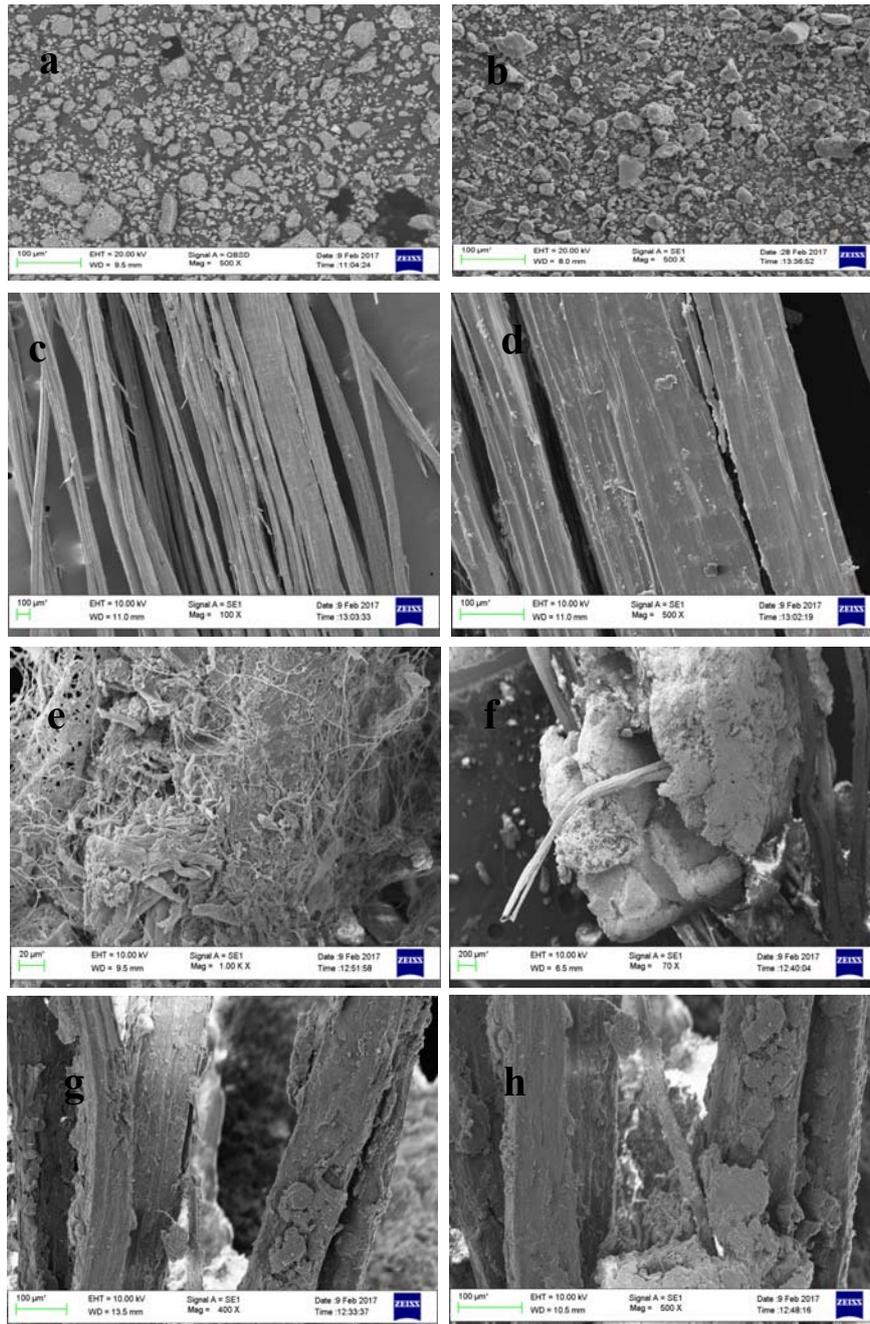
**Figure (6): SEM images (a) unreinforced silty soil with a magnification of 500X;
