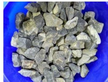
**Figure (1): Ballast material**
