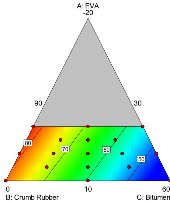
Figure (6): The contour plot for the results of phase angle for EVA/CR/bitumen mixtures
