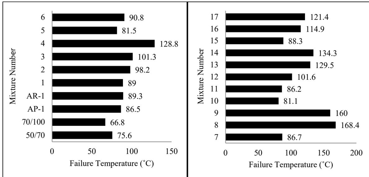
**Figure (4): Failure temperature of two penetration grade bitumens, two industrial EVA- and crumb rubber-modified bitumen samples and seventeen laboratory mixtures tested according to ASTM D7175 (ASTM D7175-15 2015)**
