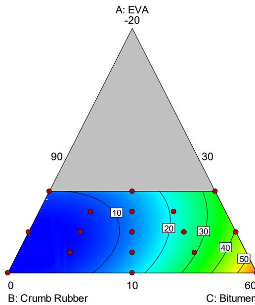
Figure (7): The contour plot for the results of rutting parameter for EVA/CR/bitumen mixtures
