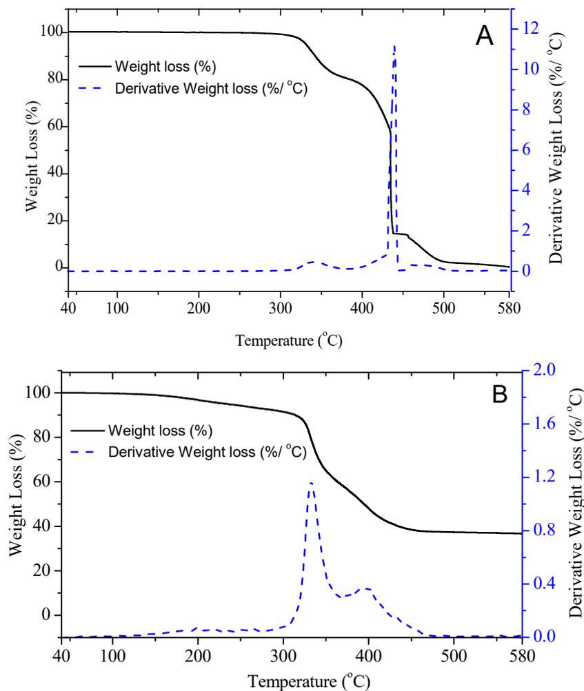
**Figure (2): Thermograms of (A) waste tyre rubber crumb 40 mesh and (B) ethylene vinyl acetate used in the EVA/CR-modified bitumen formulations**
