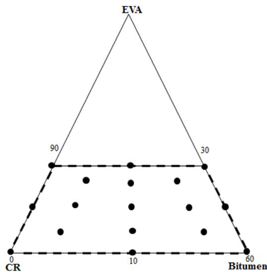
**Figure (3): The experimental runs for the three-component mixture design with upper and lower constraints for EVA, CR and bitumen**
