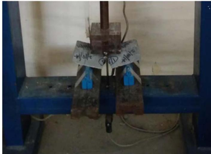
Figure (4): Flexural specimen after failure
