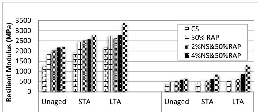
Figure (3): Resilient modulus for unaged and aged NS/PMA mixtures at 25 and 40°C
