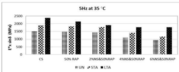
Figure (8): Fatigue factor for ageing condition
