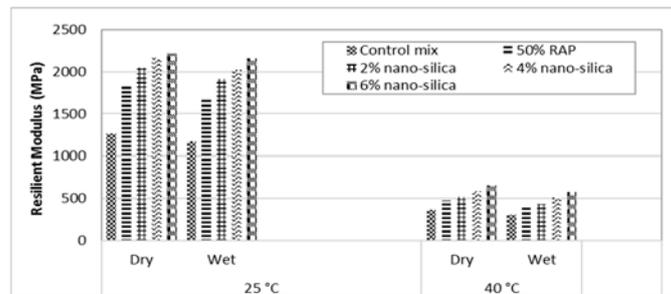
Figure (4): Resilient modulus for dry and wet NS/PMA mixtures at 25°C and 40°C
