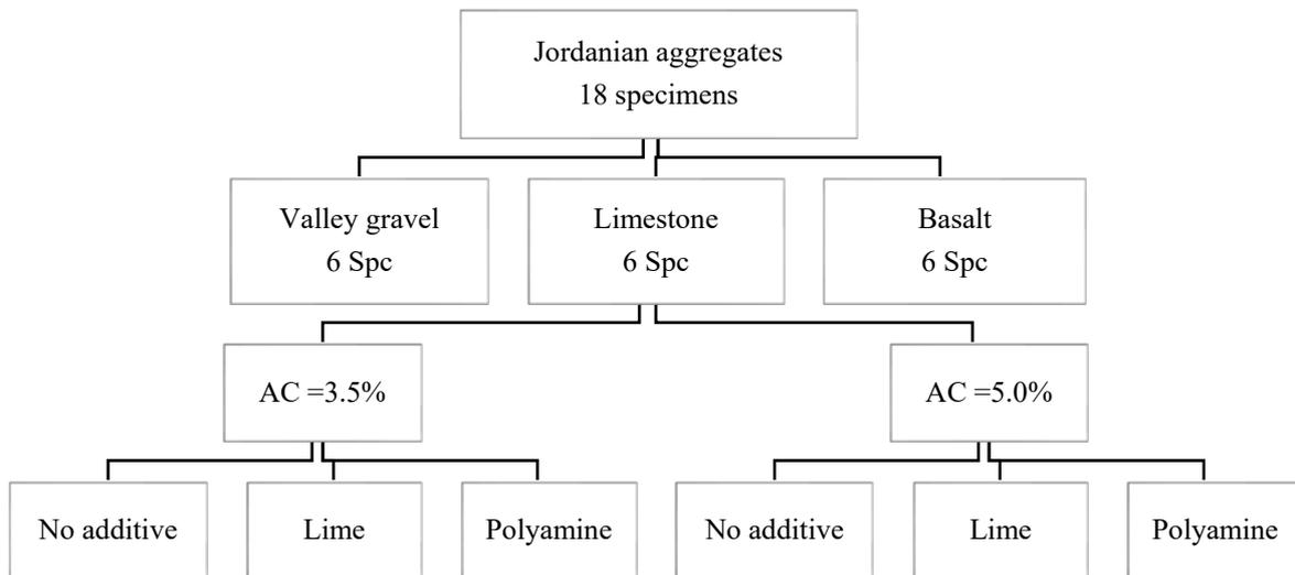
Figure (3): Flow chart for rolling bottle test
