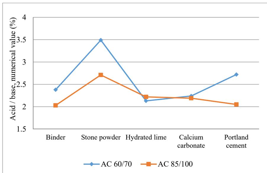
Figure (1): Numerical value of acid/base in different types of mastic and binder
