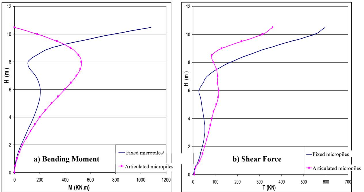
**Figure (10): Influence of micropile/shear connection on the dynamic forces in the micropiles (frictional soil ( $\phi=30^\circ$ ,  $C=2$  kPa,  $\psi=20^\circ$ ), earthquake of Turkey,  $V_g = 60$  cm/s)**
