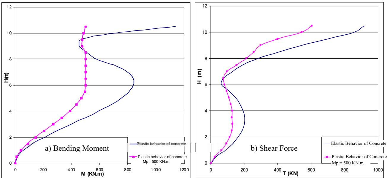
**Figure (3): Influence of nonlinear behavior of concrete pile on dynamic forces in the corner piles (frictional soil, earthquake of Turkey,  $V_g = 40$  cm/s)**
