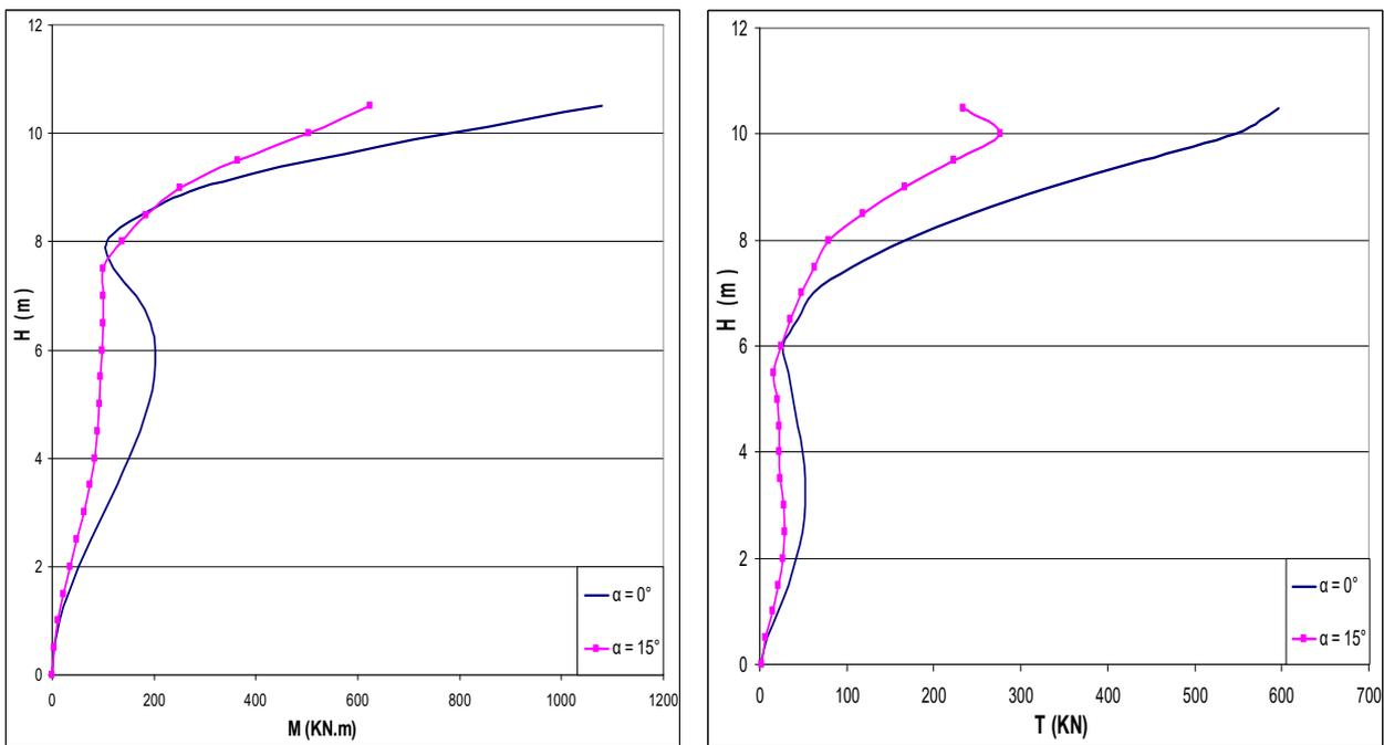
**Figure (12): Influence of inclination of the micropiles on the dynamic forces in the micropiles (frictional soil ( $\phi=30^\circ$ ,  $C=2$  kPa,  $\psi=20^\circ$ ), earthquake of Turkey,  $V_g = 60$  cm/s)**
