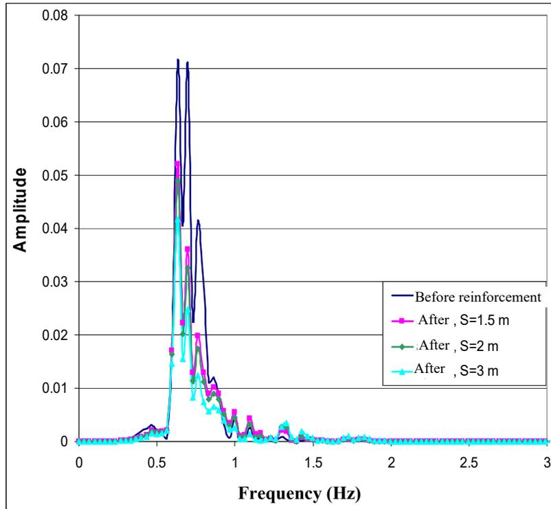
Figure (7): Influence of pile-micropile spacing on the superstructure head spectral velocity
