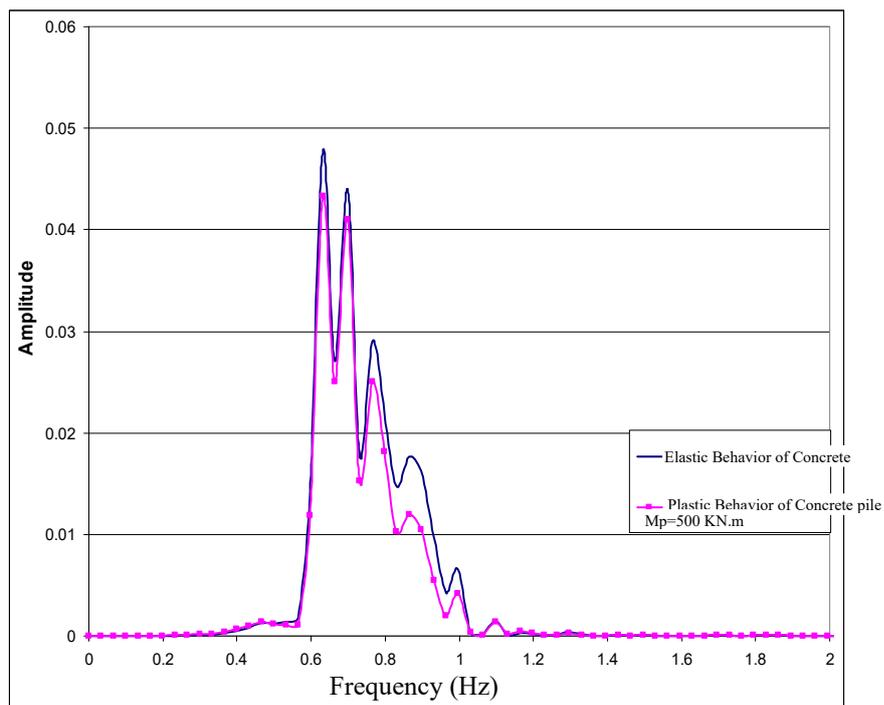
**Figure (4): Influence of nonlinear behavior of concrete pile on the superstructure head spectral velocity (Fourier spectra diagram) (frictional soil, earthquake of Turkey,  $V_g = 40$  cm/s)**
