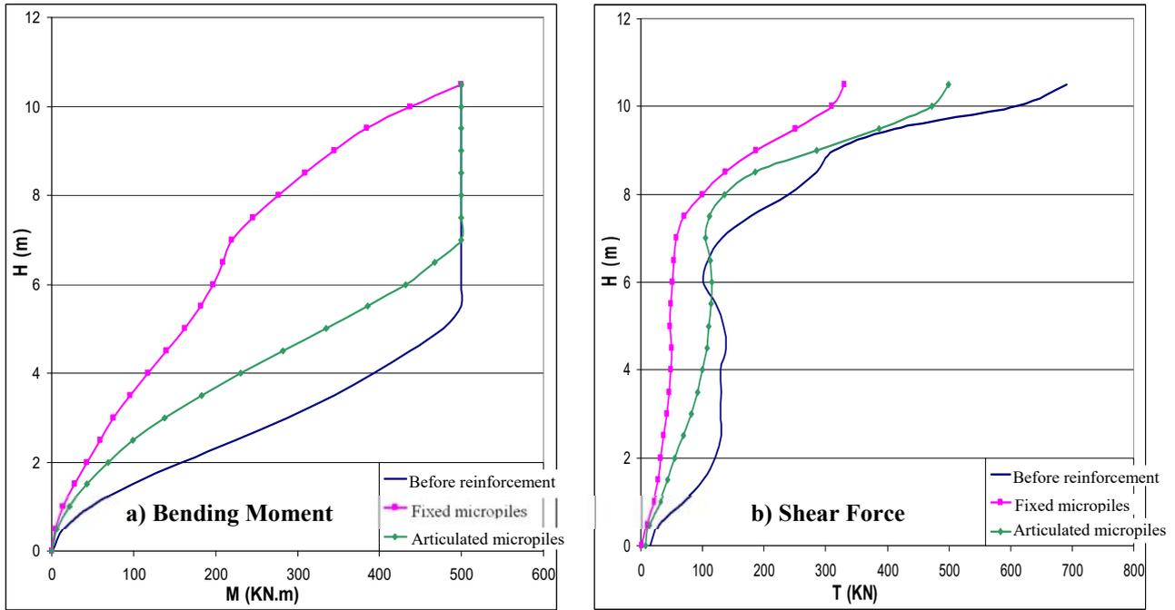
**Figure (9): Influence of micropile/shear connection on the dynamic forces in the corner piles (frictional soil ( $\phi=30^\circ$ ,  $C=2$  kPa,  $\psi=20^\circ$ ), earthquake of Turkey,  $V_g = 60$  cm/s)**
