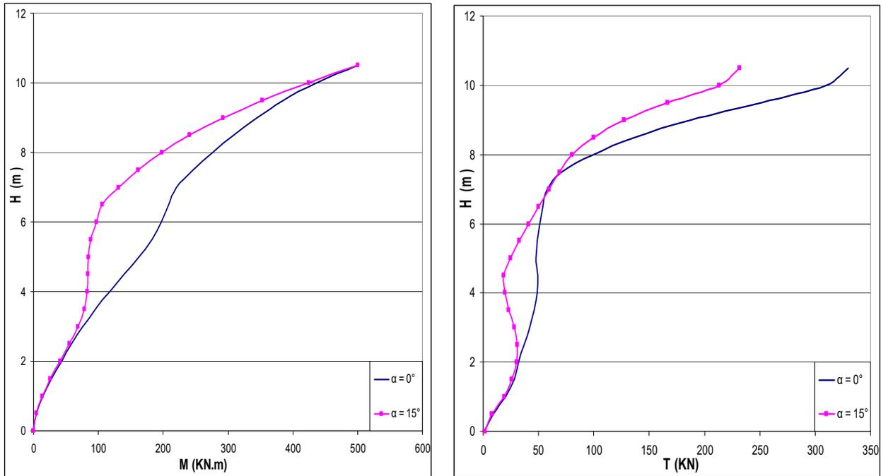
**Figure (11): Influence of inclination of the micropiles on the dynamic forces in the corner piles (frictional soil ( $\phi=30^\circ$ ,  $C=2$  kPa,  $\psi=20^\circ$ ), earthquake of Turkey,  $V_g = 60$  cm/s)**
