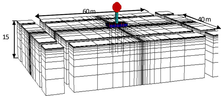
**b) 3D numerical mesh with absorbing boundaries (138 beam elements and 6978 nodes)**
