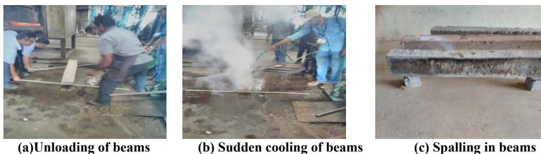
**Figure (2): Beams subjected to fire loading**
