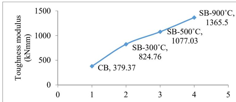
Figure (10): Comparison of toughness for beams
