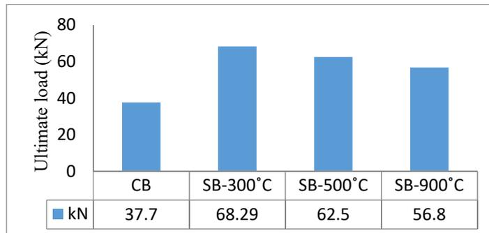
Figure (6): Comparison of ultimate load for beams
