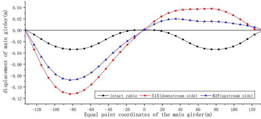
Figure (9): The influence of the downstream breaking of S15 cable on the alignment shape of the main girder
