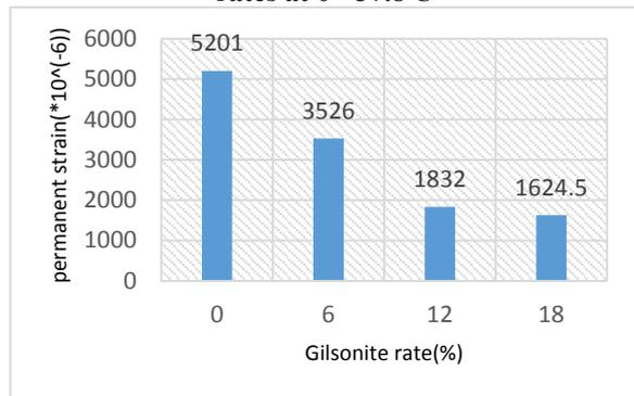
Figure (18): Change in permanent strain for optimum bitumen amounts and for certain gilsonite rates at  $\theta = 54.4^\circ\text{C}$
