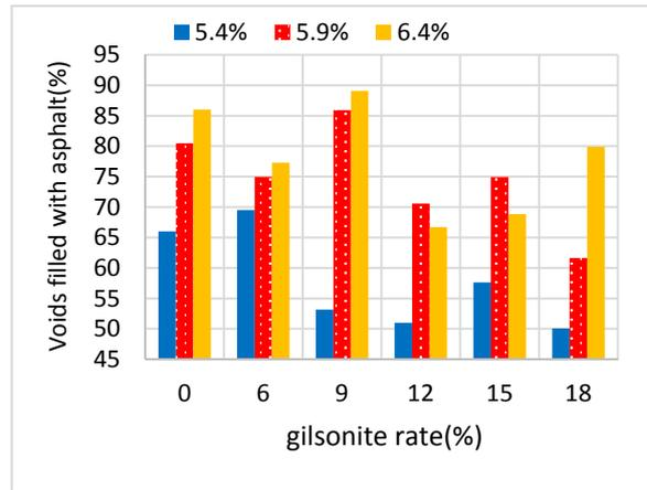
Figure (8): Change in voids filled with asphalt for different bitumen amounts and for certain gilsonite rates
