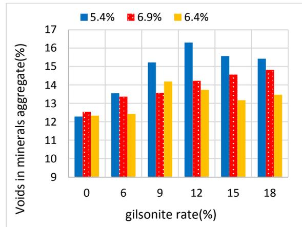
Figure (10): Change in voids in mineral aggregate for different bitumen amounts and for certain gilsonite rates
