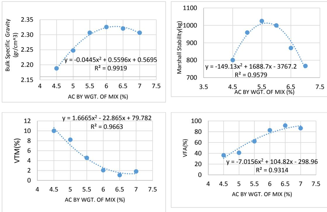
Figure (2): a) Bulk specific gravity (b) Marshall stability (c) Air voids and (d) Voids filled with asphalt
