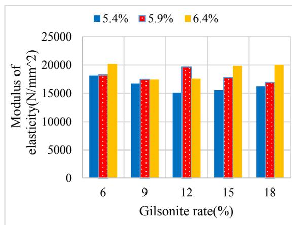
Figure (12): Change in modulus of elasticity for different bitumen amounts and for certain gilsonite rates
