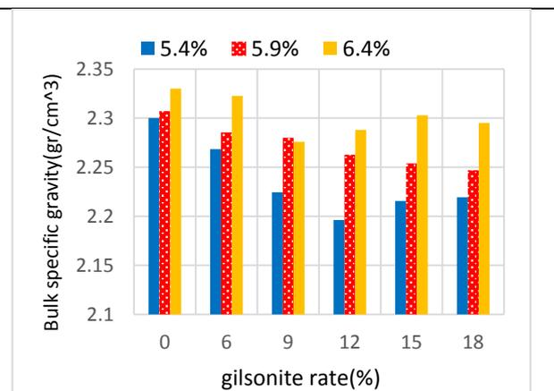
Figure (6): Change in bulk specific gravity for different bitumen amounts and for certain gilsonite rates
