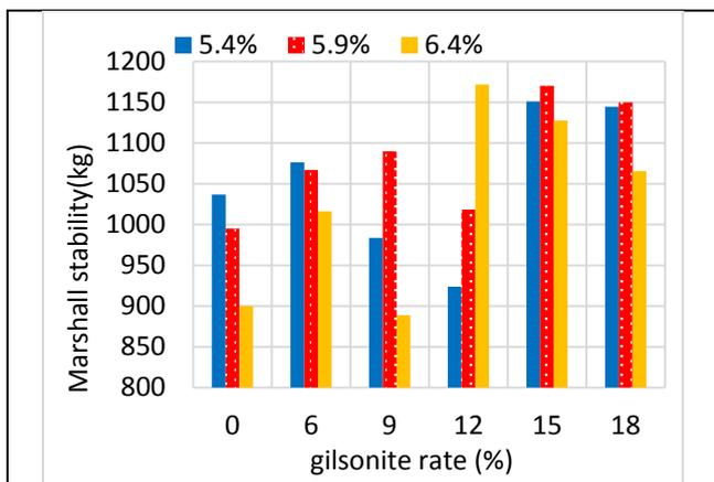
Figure (5): Change in Marshall stability for different bitumen amounts and for certain gilsonite rates
