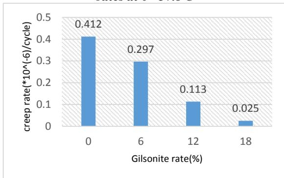
Figure (17): Change in creep rate for optimum bitumen amounts and for certain gilsonite rates at  $\theta = 54.4^\circ\text{C}$
