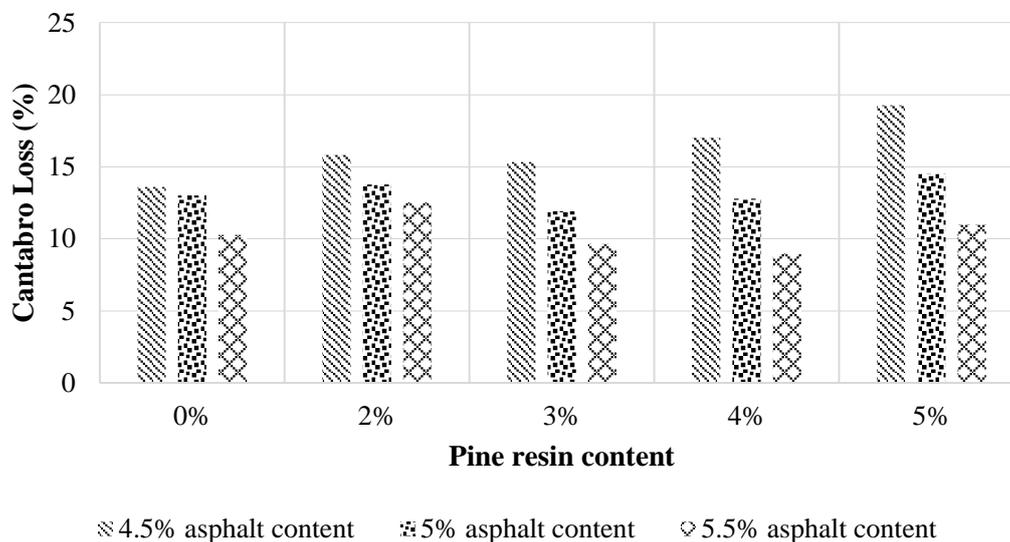
Figure (1): Cantabro loss versus pine-resin content
