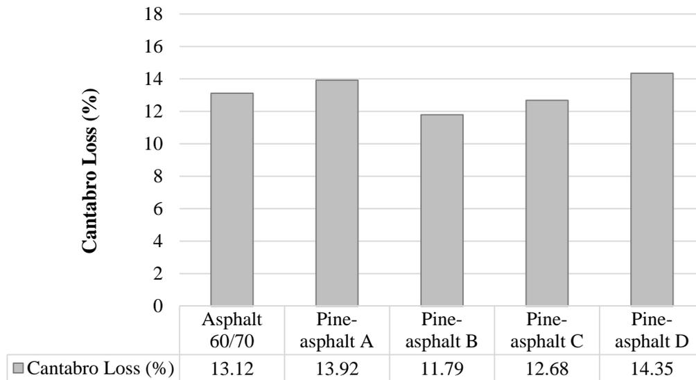
**Figure (4): Cantabro loss at optimum asphalt content**
