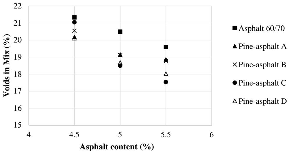
Figure (2): Voids in mix versus asphalt content
