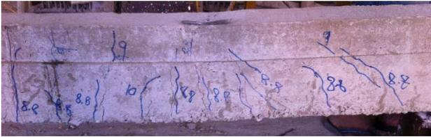
**Figure (16)(b): Cracking pattern of specimen GIM-5 (mid-span of the beam)**
