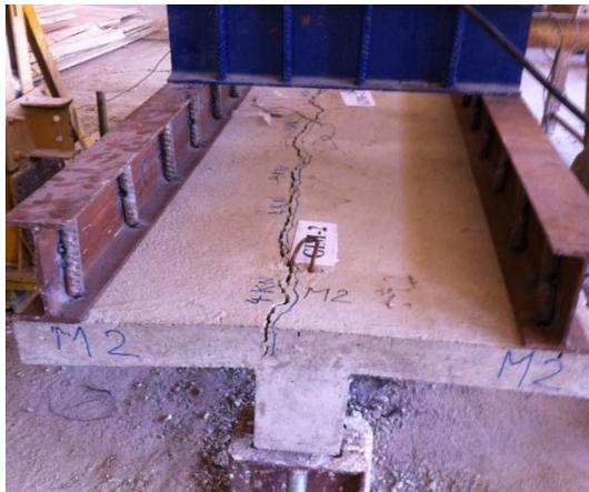
**Figure (13): Crack pattern in the slab of specimen GIM-2**
