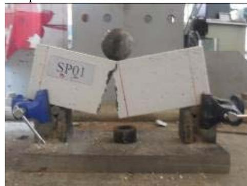
**Figure (5): Fracture of specimen SP01-B1**
