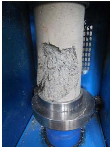
**Figure (3): Compressive test set-up**
