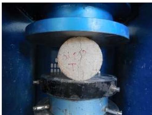
**Figure (4): Splitting tensile test setup**
