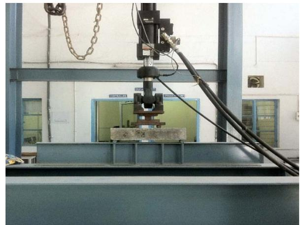
**Figure (1): Flexural strength test**
