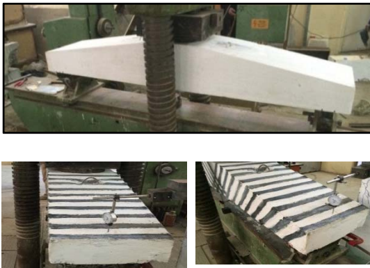
Plate (2): Test procedure for hammer head beams
