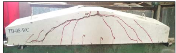
Figure (4): Crack patterns of beam specimen (TB-0S-WC)
