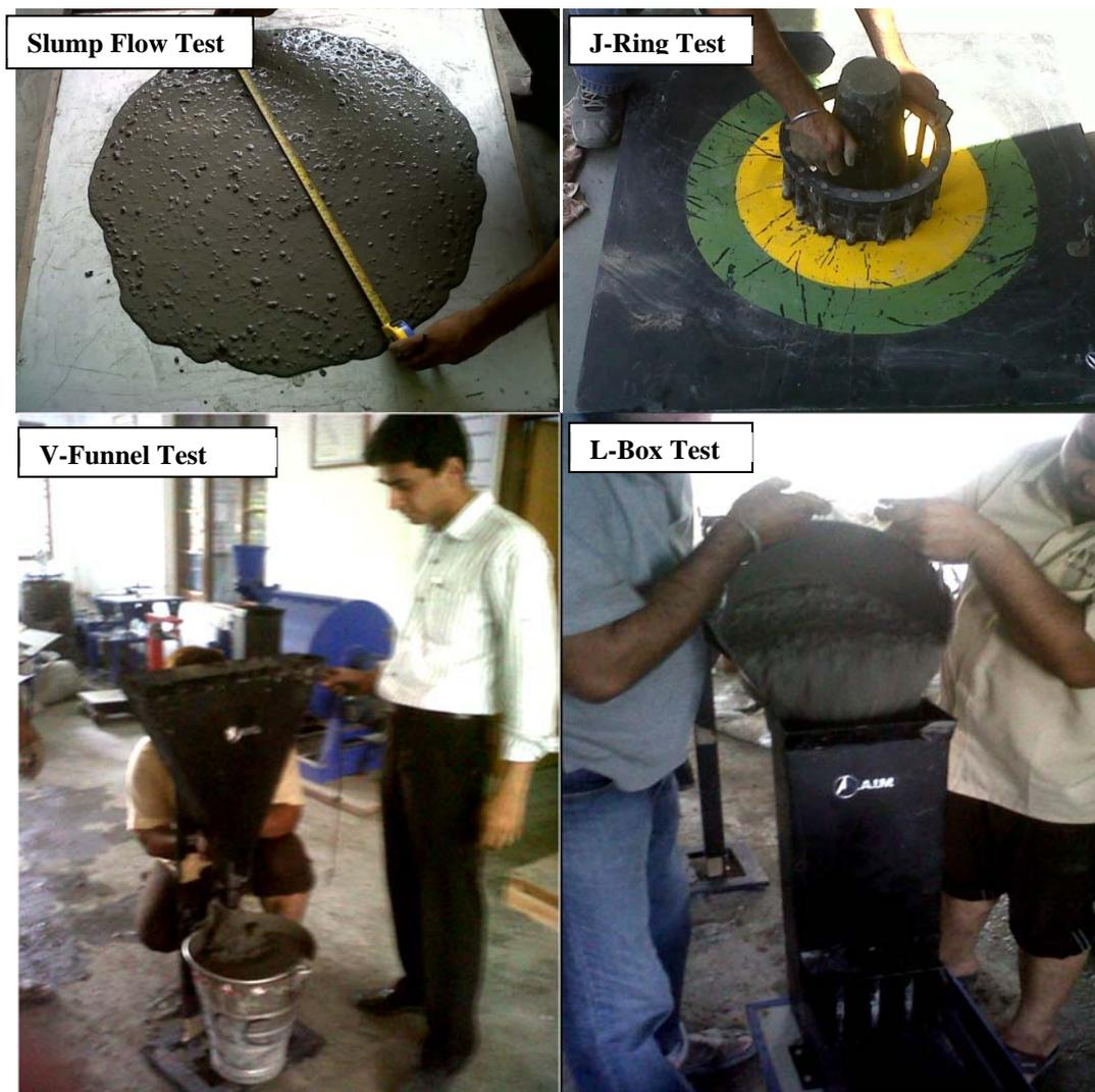
Figure (2): Workability tests conducted on SCFRC mixes
