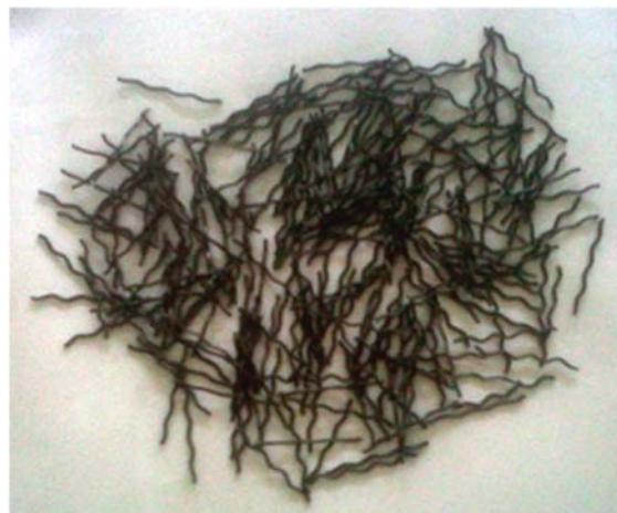
**Figure (1): Steel fibres used in the investigation**
