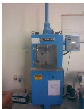
**Figure (1): Troxler model 4140 superpave gyratory compactor**
