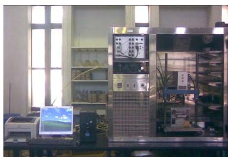
**Figure (2): Universal testing machine**
