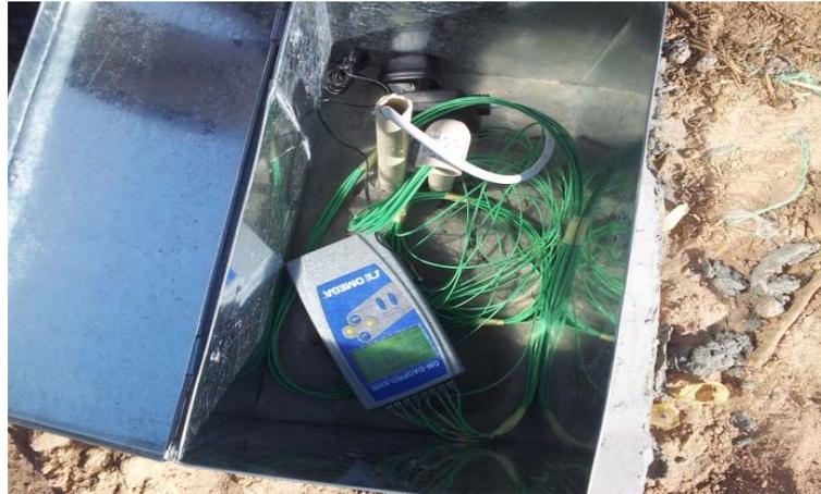
Figure (9): All of the sensors were connected to a data logger that could read and record the measured data for an entire year ( $\approx 8760$  hours)
