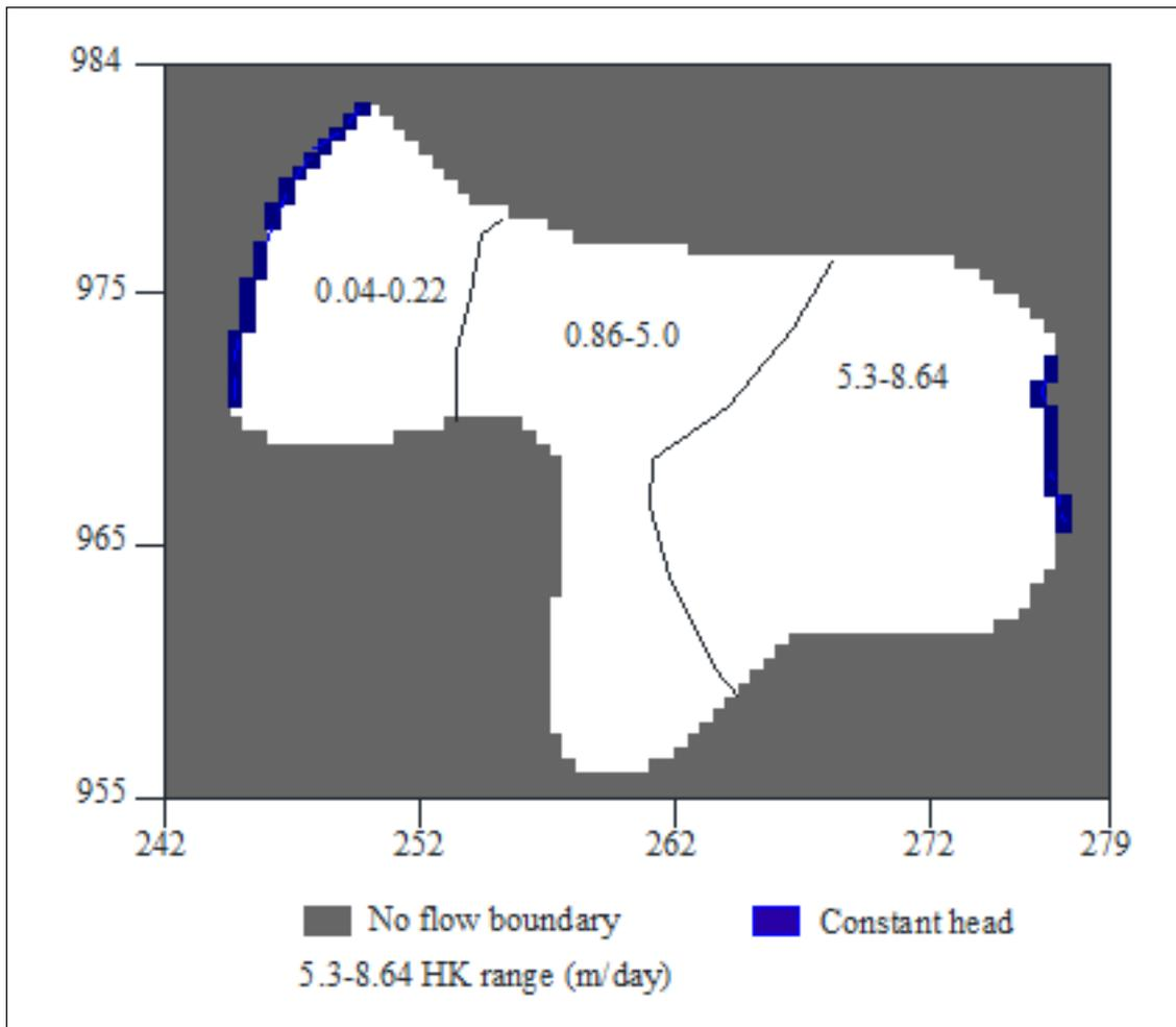
Figure (5): Map of the calibrated horizontal hydraulic conductivity of the B4 formation system
