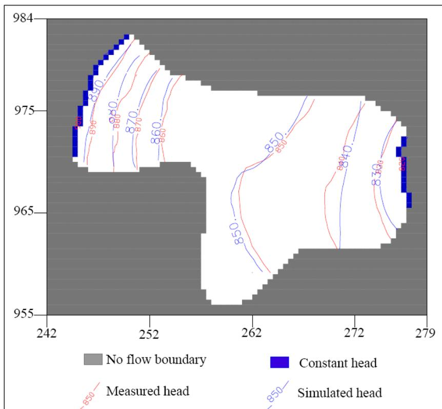
Figure (4): Map of the measured and simulated water levels for the B4 formation (steady state calibration)
