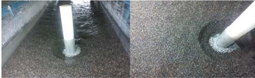
**Figure (12): A view of scour hole protected by nano-clay material**
