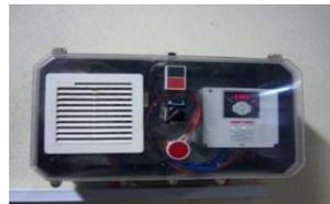
Figure (2): Frequency-adjusting device used to control flow rate
