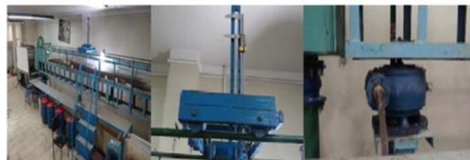
Figure (3): A. Channel used in experiment; B. Digital level gauge; C. Hydraulic jack
