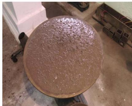
**(a) Slump flow test**
