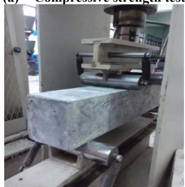
(c) Flexural strength test
