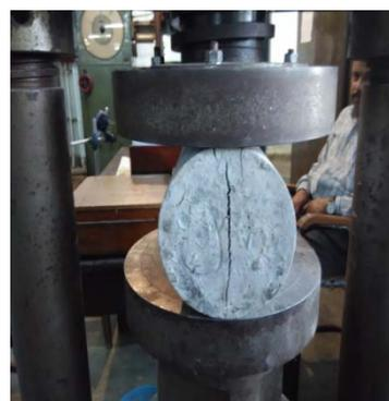
(b) Splitting tensile strength test
