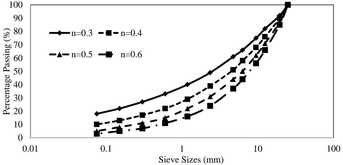
Fig.1: Gradation curves for UGMs
