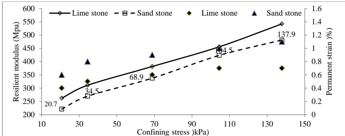
Fig.3: Effect of Confining Stress on Resilient Modulus and Permanent Strain
