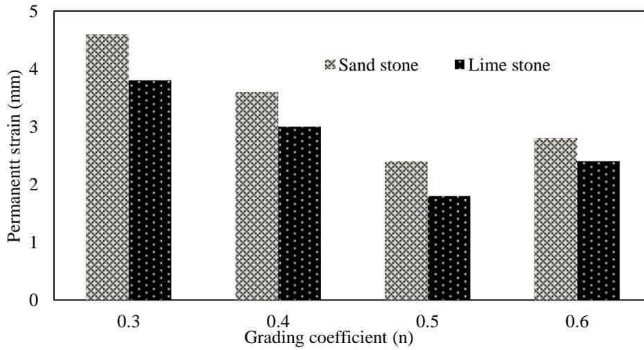
Fig.5b: Effect of Aggregate type on Permanent Strain
