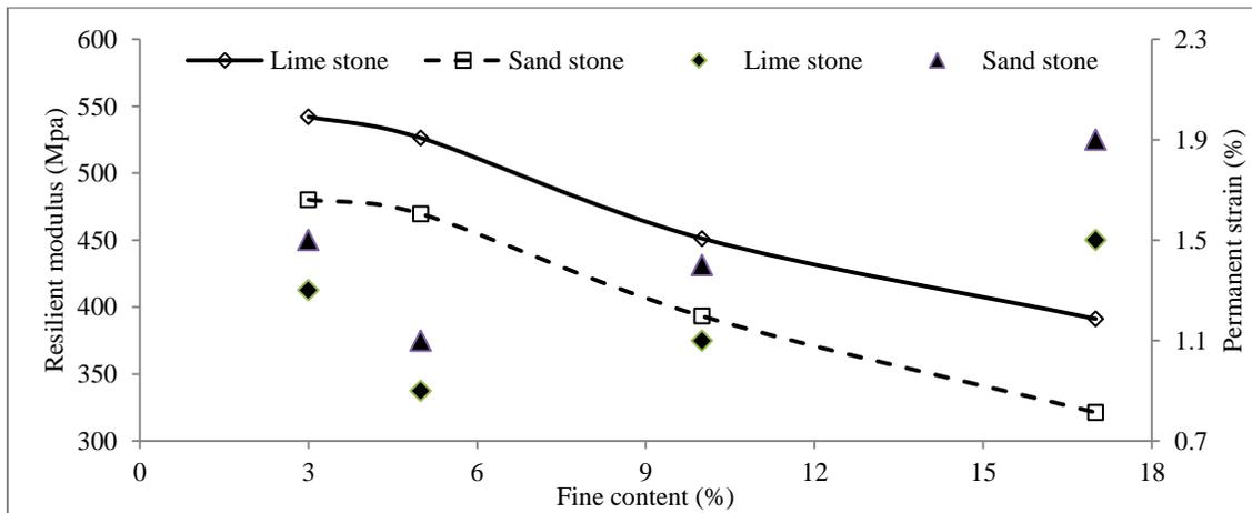
Fig.4: Effect of Fines on Resilient Modulus and Permanent Strain
