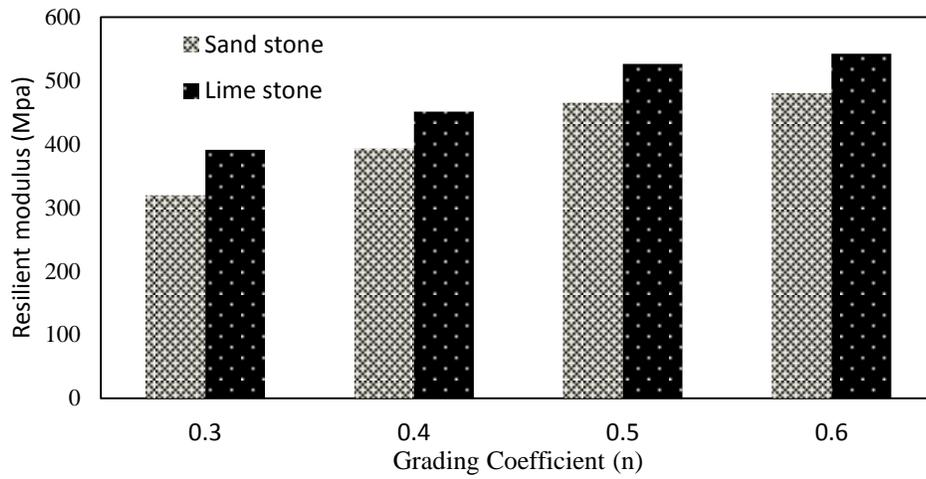
Fig.5a: Effect of Aggregate type on Resilient Modulus
