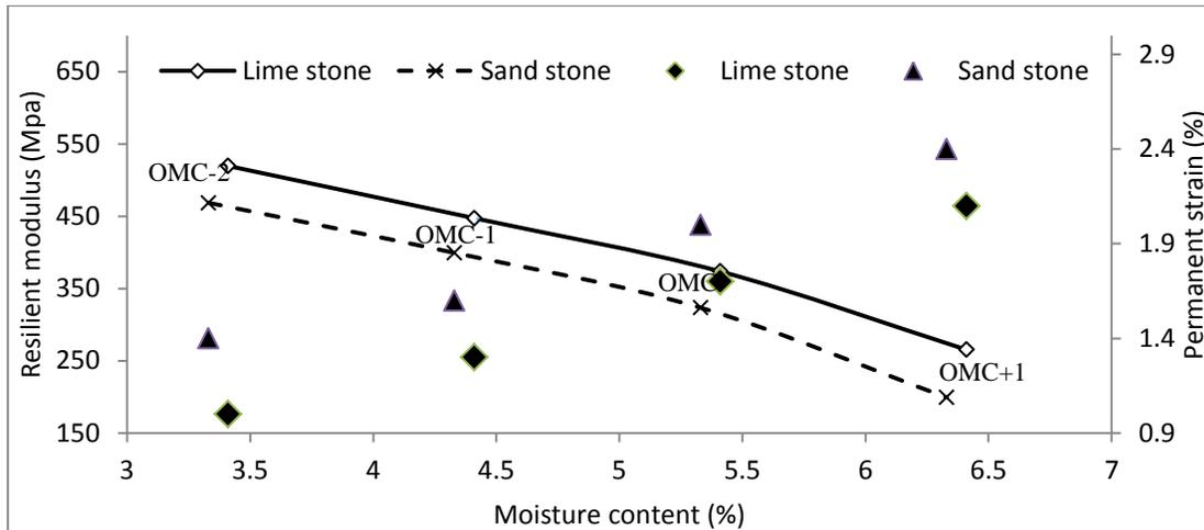
Fig.2: Effect of Moisture on Resilient Modulus and Permanent Strain
