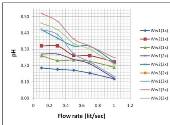
Figure (8): Relationship between pH and flow rate
