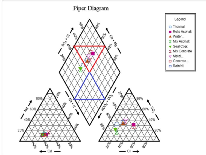
Figure (8): Piper diagram for roofing runoff water samples in the study area
